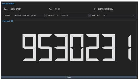
Before editing the personal ID number, the user needs to use the MX USB PG-ISP to connect the receiver and GUI, as shown in Figure 3.
